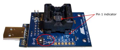
The K1 switch on the Atmel AT88CK101BK8 board should always be in the "uBase" position when
