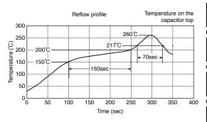
Above "Reflow Profile" graph indicates temperature at the terminals and capacitor top.
