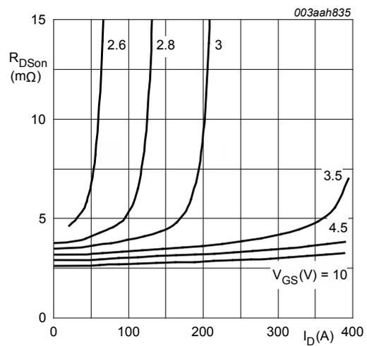
$T_j = 25\text{ }^\circ\text{C}; t_p = 300\text{ }\mu\text{s}$
