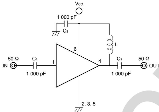
**COMPONENTS OF TEST CIRCUIT FOR MEASURING ELECTRICAL CHARACTERISTICS EXAMPLE OF ACTUAL APPLICATION COMPONENTS**
