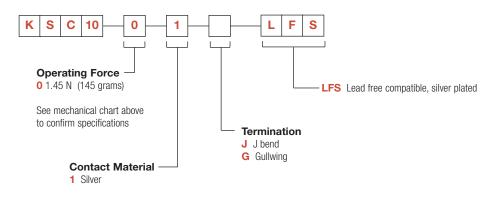
Note: KSC10 offered with yellow actuator as standard, hardness 55 Shore
