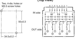
Note: Do not reverse the coil polarity.
