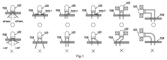
"  $\bigcirc$  " Correct mounting method "imes" Incorrect mounting method
