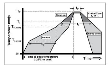
Wave Soldering Parameters
