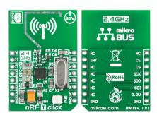
nRF T Click™ is an add-on board in mikroBUS™ form factor. It's a compact and easy solution for adding 2.4 GHz transceiver to your design. It features nRF24L01P 2.4 GHz transceiver module with an embedded baseband protocol engine as well as 2.4 GHz PCB trace antenna. nRF T Click™ communicates with target board microcontroller via mikroBUS" SPI (SDI, SDO, SCK, CS#), CE and INT lines. The board is designed to use 3.3V power supply only. LED diode (Green) indicates the presence of power supply.
