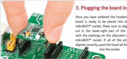
Once you have soldered the headers your board is ready to be placed into desired mikroBUS™ socket. Make sure to align the cut in the lower-right part of the board
