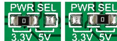
Nano GPS click features an SMD jumper [zero ohm resistor] that let's you switch between a 3.3V or a 5V power supply.
