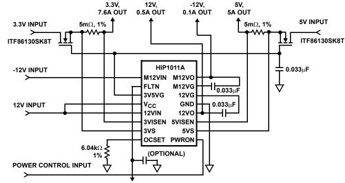
NOTE: All capacitors are  $\pm 10\%$ . FAULT OUTPUT (ACTIVE LOW)
