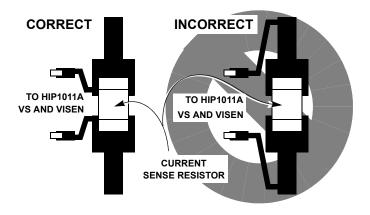
FIGURE 13. SENSE RESISTOR LAYOUT
