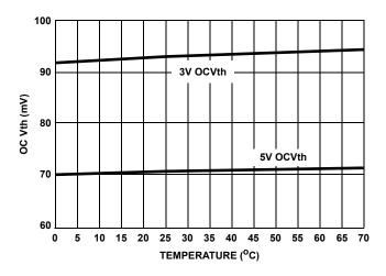
FIGURE 4. OC Vth vs TEMPERATURE (VR<sub>OCSET</sub> = 1.21V)
