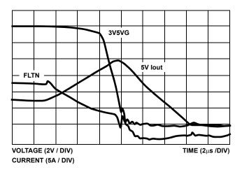
FIGURE 8. FLTN, 3V5VG RESPONSE TO OC, FLTN CAP = 0.01  $\mu\text{F}$
