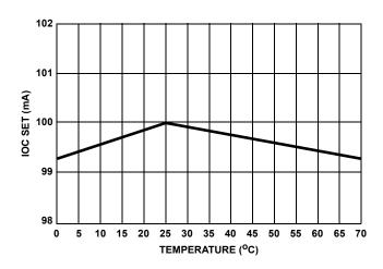
FIGURE 5. OCSET I vs TEMPERATURE
