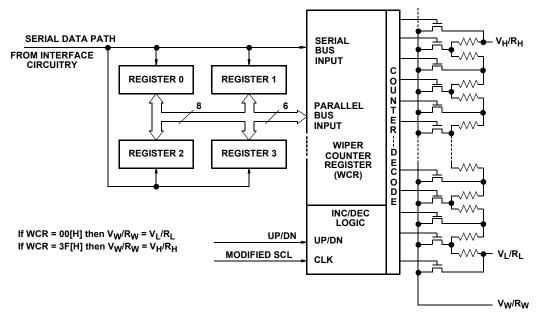
FIGURE 12. DETAILED POTENTIOMETER BLOCK DIAGRAM
