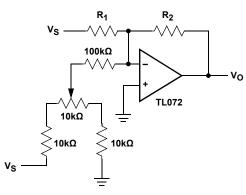
FIGURE 17. OFFSET VOLTAGE ADJUSTMENT
