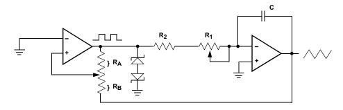
$\begin{array}{l} \text{frequency} \propto \text{R}_{1}, \, \text{R}_{2}, \, \text{C} \\ \text{amplitude} \propto \text{R}_{A}, \, \text{R}_{B} \end{array}$
