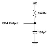
FIGURE 2. EQUIVALENT A.C. LOAD CIRCUIT
