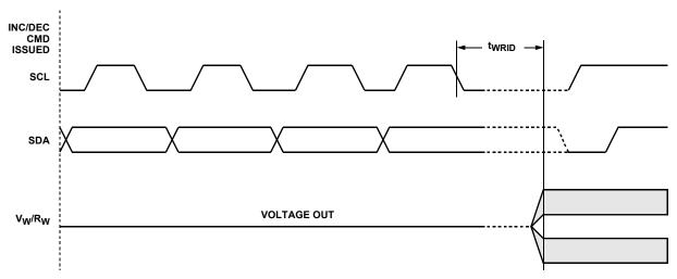
FIGURE 10. INCREMENT/ DECREMENT TIMING LIMITS
