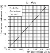
Continuous load current vs. On-state voltage On-state resistance vs. Ambient temperature
