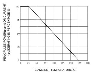
Fig. 2-PULSE DERATING CURVE
