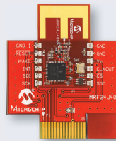
MRF24J40MA PICtail Plus 2.4 GHz RF Card (AC164134)
