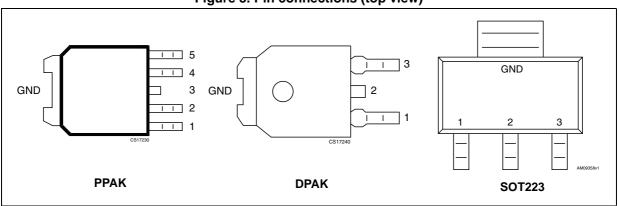
Figure 3. Pin connections (top view)
