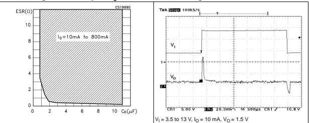
Figure 19. Load transient
