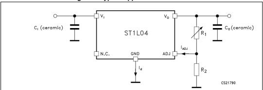
The adjustable output voltage is set by a resistor divider connected between  $V_O$  and GND with its centre tap connected to ADJ. The voltage divider resistors are: R1 connected between  $V_O$  and ADJ and R2 connected between ADJ and GND.  $V_O$  is given by  $V_{REF}$ ,  $R_1$ ,  $R_2$ ,  $I_{ADJ}$ , as follows:
