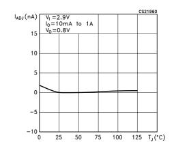
Figure 19. Minimum output current for regulation vs. temperature V<sub>i</sub>= 5.5 V
