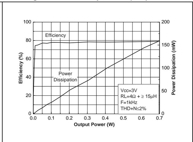
Figure 10. Efficiency vs. output power
