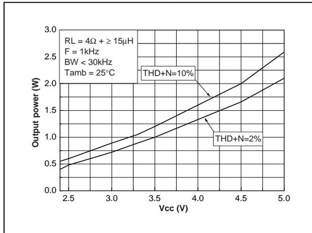
Figure 13. Output power vs. power supply voltage
