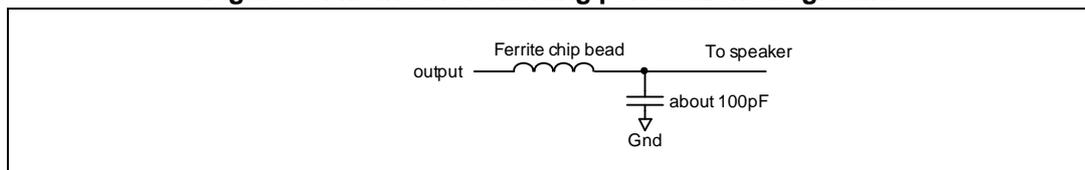
In the case where the distance between the A21SP16 outputs and speaker terminals is high, it is possible to have low frequency EMI issues due to the fact that the typical operating frequency is 250 kHz. In this configuration, we recommend using an output filter (as shown
