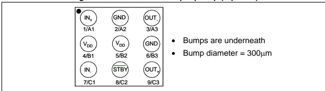
**Figure 68. Marking for 9-bump flip-chip (top view)**
