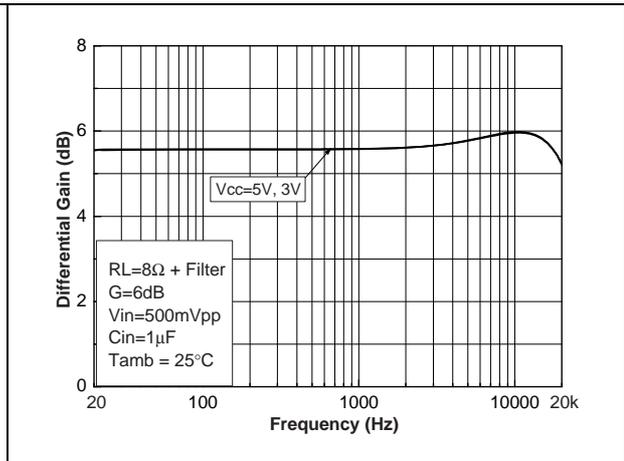
Figure 54. Gain vs. frequency
