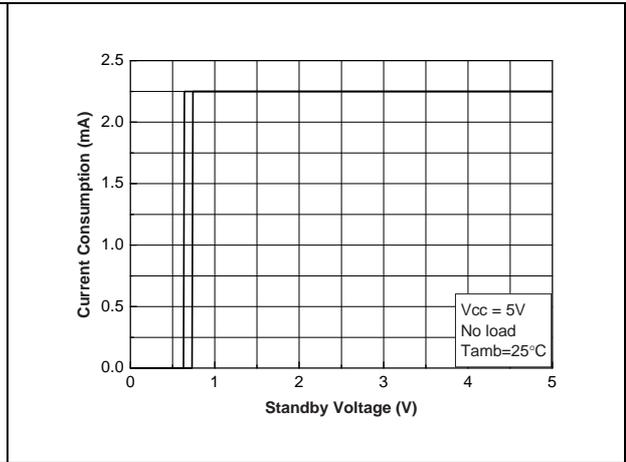
Figure 6. Current consumption vs. standby voltage
