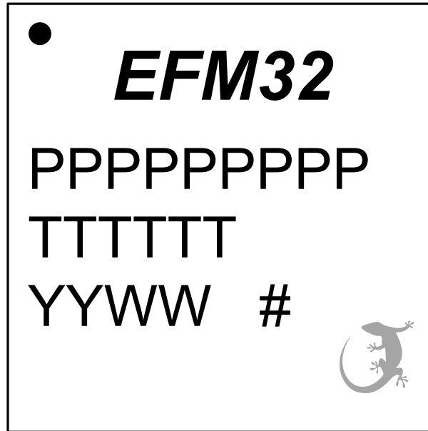
Figure 8.3. QFN32 Package Marking
