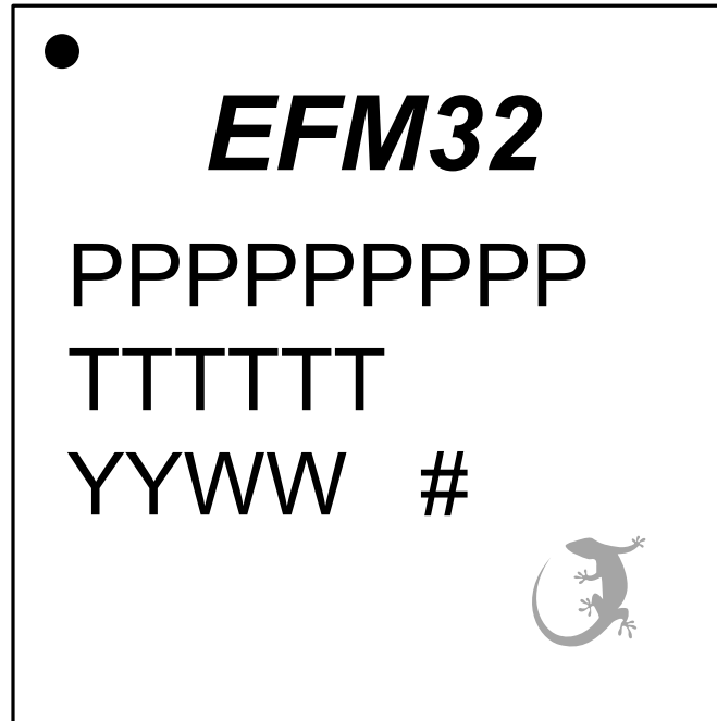
Figure 7.3. QFN48 Package Marking
