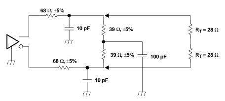
Figure 1. Test Load and Voltage Definitions ( $V_{O(STOP)}$ ,  $V_{O(X)}$ ,  $V_{O}$ ,  $V_{OH}$ ,  $V_{OL}$ )
