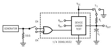
C<sub>L</sub> includes load and test jig capacitance.
