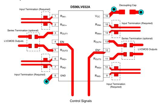
Figure 11. DS90LV032A Layout Example
