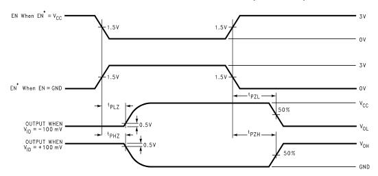
Figure 7. Receiver TRI-STATE Delay Waveforms
