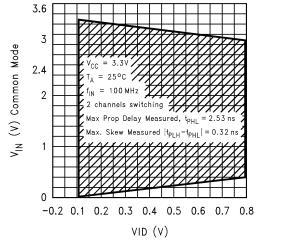
Figure 10. Typical Common Mode Range Variation With Respect to Amplitude of Differential Input
