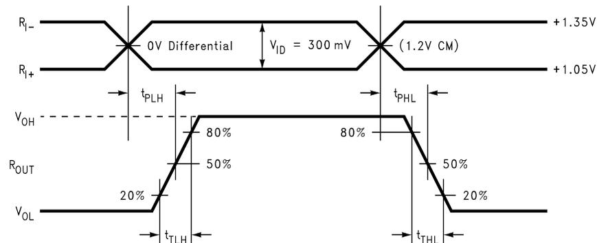
Figure 9. Receiver Propagation Delay and Transition Time Waveforms
