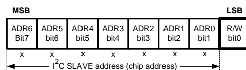
Figure 18. I²C Chip Address
