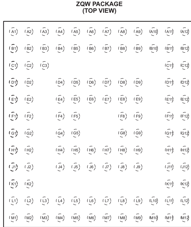
Figure 4-3. 113-Pin ZQW Package (Top View) – MSP430F6438, MSP430F6436, MSP430F6435, MSP430F6433
