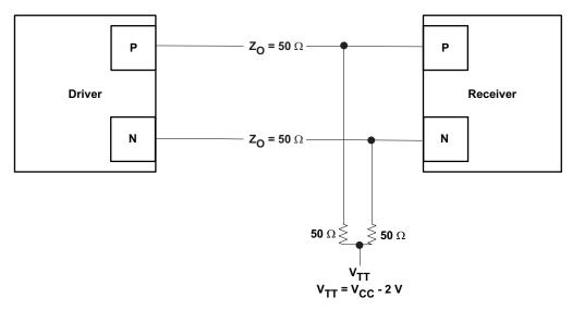
Figure 1. Termination for Output Driver
