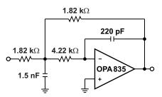
Figure 78. MFB 100-kHz Second-Order Low-Pass Butterworth Filter Circuit
