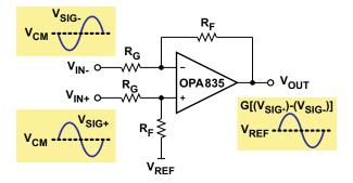
Figure 67. Differential to Single-Ended Amplifier
