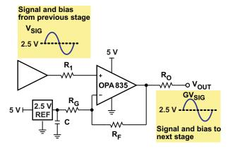
Figure 60. Noninverting Single Supply With Reference
