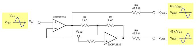
Figure 66. Cat5 Line Driver With Gain = 2 V/V (6 dB)
