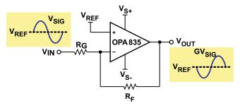
Figure 54. Inverting Amplifier
