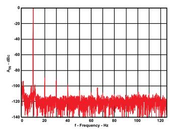
Figure 73. ADS8326 and OPA835 10-kHz FFT
