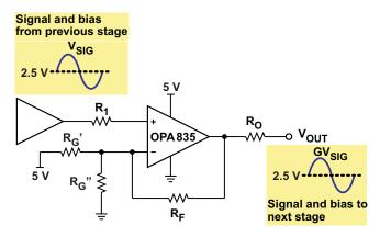
Figure 61. Noninverting Single Supply With Resistors
