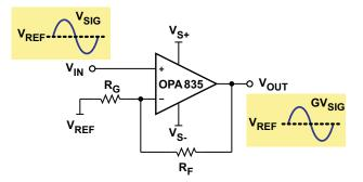
Figure 53. Noninverting Amplifier
