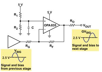
Figure 63. Inverting Single Supply With Resistors
