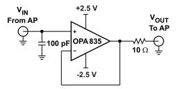
The 100-pF capacitor to ground on the input helped to decouple noise pick up in the lab and improved noise performance.
