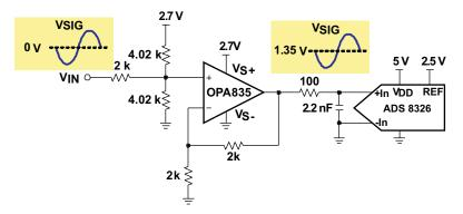
Figure 72. OPA835 and ADS8326 Test Circuit
