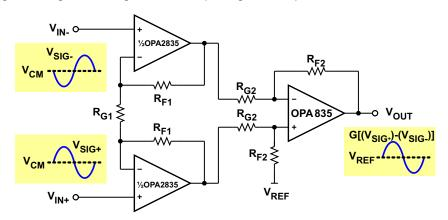
Figure 64. Instrumentation Amplifier
