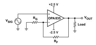
Figure 58. Split-Supply Operation
