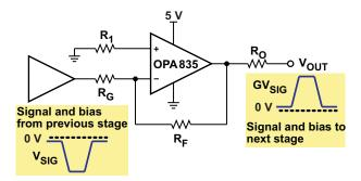
Figure 71. Inverting Single Supply With Pulse
