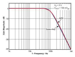
Figure 80. MFB and Sallen-Key Second-Order Low-Pass Butterworth Filter Response
