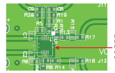
Dark green areas indicate regions of the PCB where the underlying Ground and Power Planes have been removed in order to minimize parasitic capacitance on the sensitive input and output nodes.
