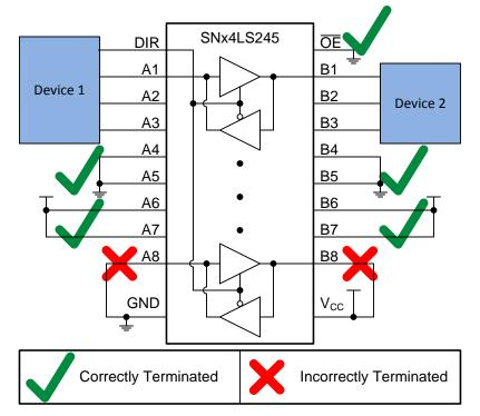
Figure 7. Example Demonstrating How to Terminate Unused Inputs and Channels of a Transceiver
