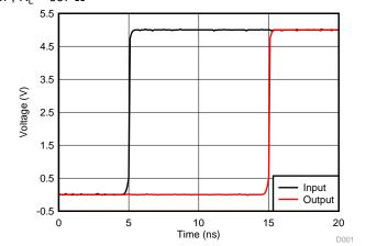
Figure 1. Simulated Propagation Delay From Input to Output
