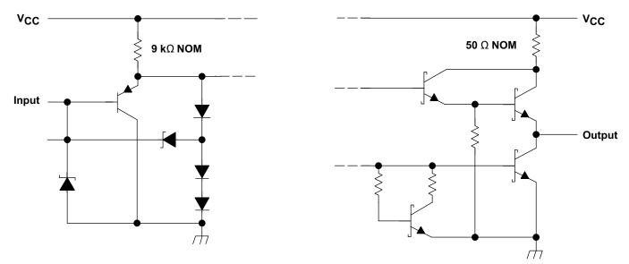
Figure 4. Schematics of Inputs and Outputs
