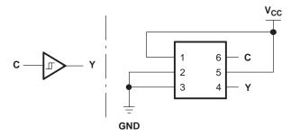
Figure 8. Noninverted Buffer
