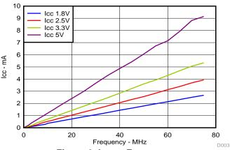
Figure 6. I<sub>CC</sub> vs Frequency
