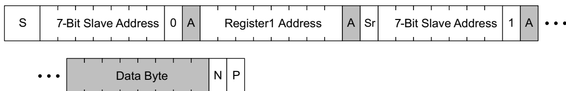
Figure 30. I²C Read Data Format
