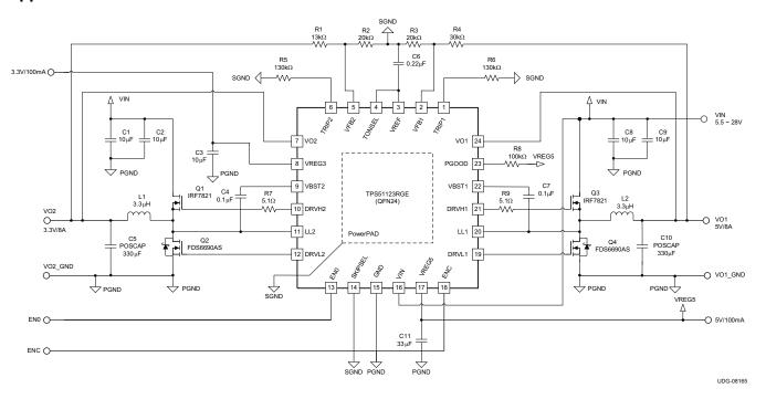
Figure 39. 5-V/8-A, 3.3-V/8-A Application Circuit (245-kHz/305-kHz Setting)
