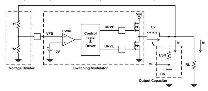
Figure 36. Simplifying the Modulator
