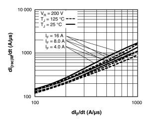
Fig. 8 - Typical dl<sub>(rec)M</sub>/dt vs. dl<sub>F</sub>/dt (Per Leg)
