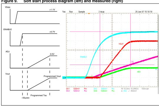
Figure 9. Soft start process diagram (left) and measured (right)
