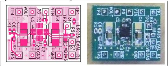
Different values for  $R_1$  are available in order to program the value of  $V_{OUT}$  ( $R_2$  = 10 k $\Omega$ )
