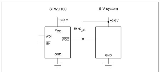
Figure 4: Open drain WDO output connection
