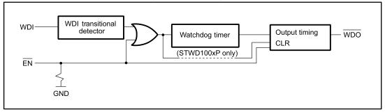
Figure 3: Block diagram
