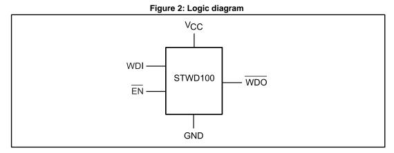
1. The WDO output is available in open drain or push-pull configuration.
