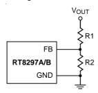
Figure 1. Output Voltage Setting
