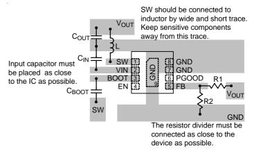
Figure 4. PCB Layout Guide
