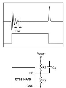
Figure 1. Cff Capacitor Setting
