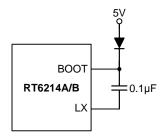
Figure 6. External Bootstrap Diode
