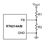
Figure 5. Output Voltage Setting
