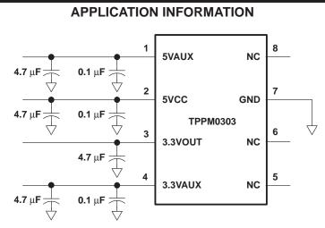
Figure 11. Typical Application Schematic
