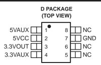
The TPPM0303 is a low-dropout regulator with auxiliary power management that provides a constant 3.3-V supply at the output capable of driving a 250-mA load.
