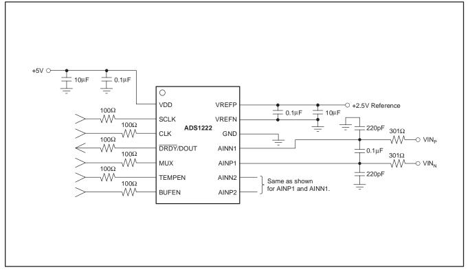
Figure 30. Basic Connections
