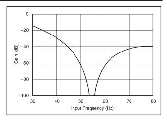
Figure 22. Frequency Response Near 50Hz and 60Hz with  $f_{\mbox{CLK}}$  = 910kHz
