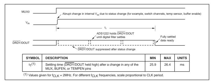
Figure 23. Example of Settling Time After Changing the Input Multiplexer
