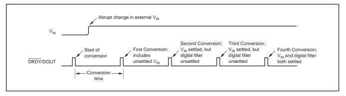
Figure 24. Settling Time in Continuous Conversion Mode
