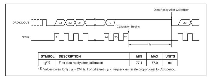
Figure 27. Self-Calibration Timing
