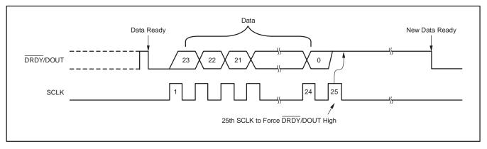
Figure 26. Data Retrieval with DRDY/DOUT Forced High Afterwards
