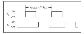
Figure 15. S<sub>1</sub> and S<sub>2</sub> Switch Timing for Figure 14
