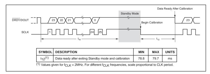
Figure 29. Standby Mode with Self-Calibration Timing (can be used for single conversions)
