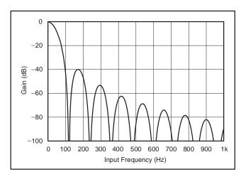
Figure 21. Frequency Response to 1kHz
