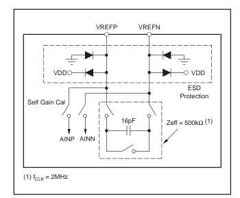
Figure 19. Simplified Reference Input Circuitry
