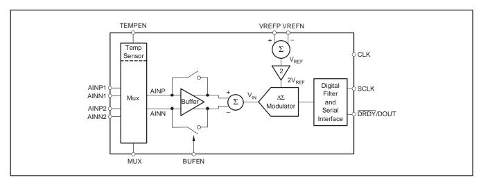
Figure 13. Conceptual Diagram of the ADS1222
