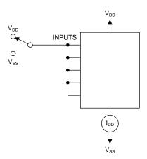
Figure 14. Quiescent Device Current Test Circuit
