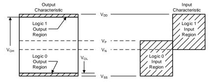
Figure 12. Input and Output Characteristics
