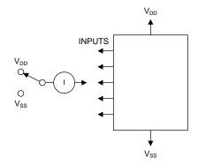
Figure 15. Input Current Test Circuit
