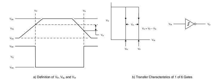
Figure 13. Hysteresis Definition, Characteristics, and Test Set-Up
