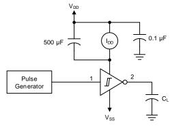
Figure 16. Dynamic Power Dissipation Test Circuit
