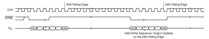
Figure 50. SYNC Interrupt Facility
