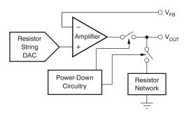
Figure 48. Output Stage During Power-Down
