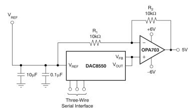
Figure 51. Bipolar Output Range
