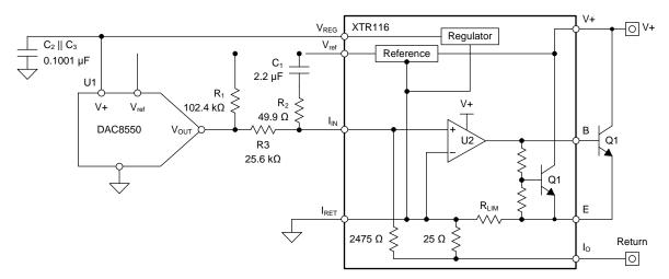
Figure 52. Loop-Powered Transmitter
