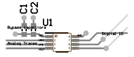
Figure 59. Layout Diagram
