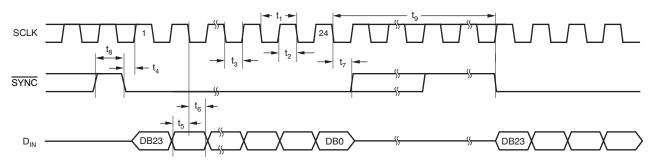
Figure 1. Serial Write Operation
