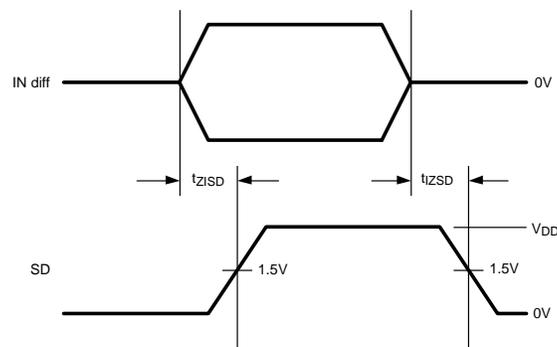
Figure 4. Signal Detect (SD) Delay Timing Diagram
