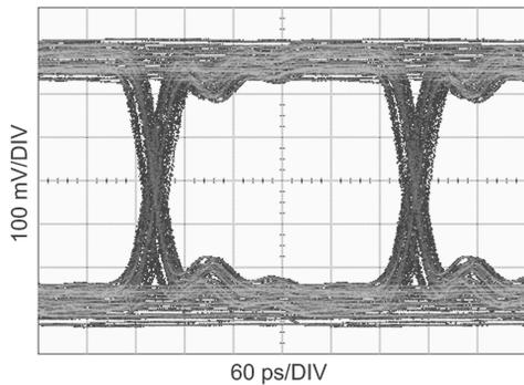
Figure 14. Equalized Signal (32 In Tyco XAUI Backplane, 3.125 Gbps, PRBS7, 0x07 Setting)
