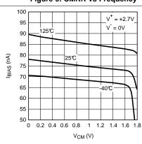
Figure 11. Input Bias Current vs V<sub>CM</sub>
