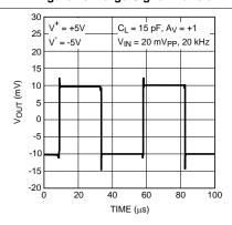
Figure 29. Small-Signal Transient Response
