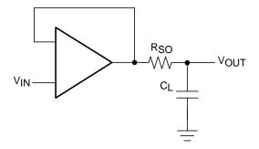
Figure 38. Compensation by Isolation Resistor
