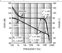
Figure 15. Open-Loop Gain and Phase With Resistive Load
