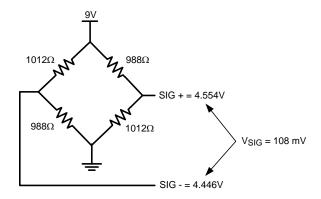
Figure 44. Sensor Output with No Load
