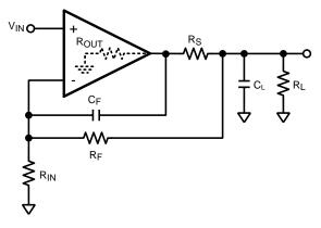
Figure 37. In the Loop Compensation
