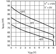
Figure 12. Input Bias Current vs V<sub>CM</sub>
