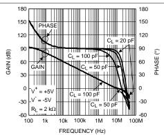
Figure 13. Open-Loop Gain and Phase With Capacitive Load
