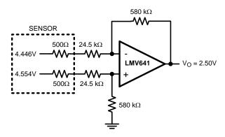
Figure 45. Thevenin Equivalent Showing Required Gain
