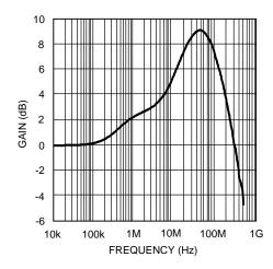
Figure 41. Equalizer Frequency Response
