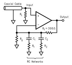
Figure 38. Equalizer Circuit Schematic
