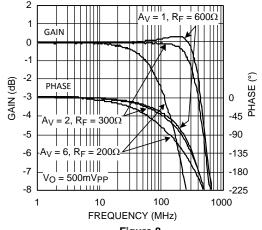
Figure 8. **Inverting Frequency Response**
