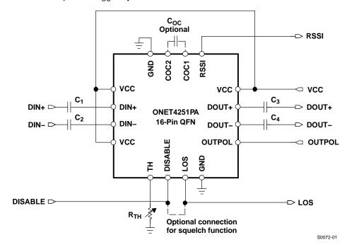
Figure 15. Basic Application Circuit With AC Coupled I/Os
