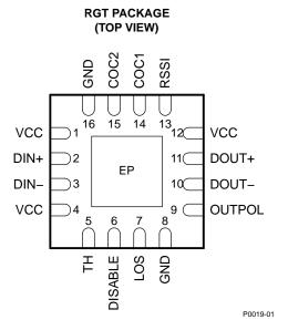
Figure 2. Pinout of ONET4251PA in a 3 mm x 3 mm 16-Pin QFN Package (Top View)
