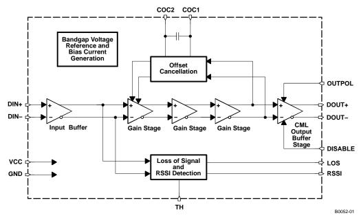
Figure 1. Simplified Block Diagram of the ONET4251PA
