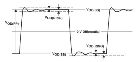
$V_{OD(RING)}$  is measured at four points on the output waveform, corresponding to overshoot and undershoot from the  $V_{OD(H)}$  and  $V_{OD(L)}$  steady state values.
