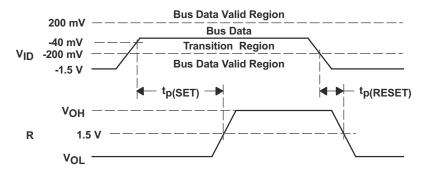
Figure 23. Receiver Active Failsafe Definitions and Waveforms
