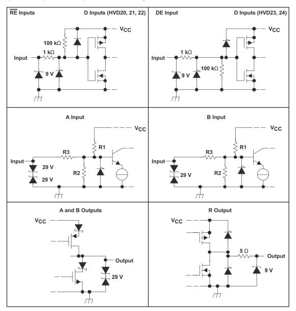
Figure 28. Equivalent Input and Output Schematic Diagrams
