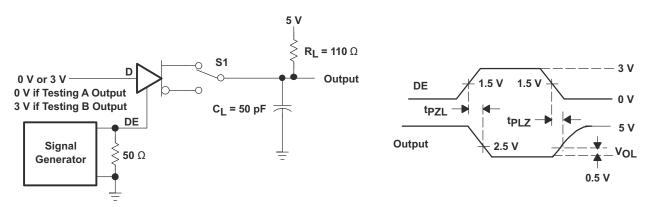
Figure 15. Driver Enable and Disable Test, Low Output
