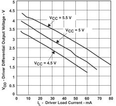
Figure 4. Driver Differential Output Voltage vs Driver Load Current
