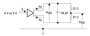
Figure 9. Driver Test Circuit, V<sub>OD</sub> and V<sub>OC</sub> Without Common-Mode Loading
