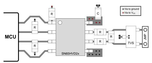
Figure 32. SN65HVD2x Layout Example
