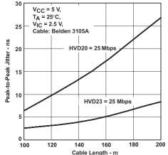
Figure 6. SN65HVD2[0,3] Peak-to-Peak Jitter vs Cable Length
