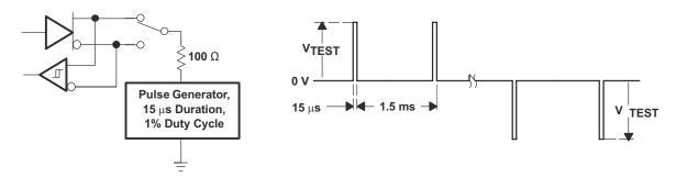
Figure 24. Test Circuit and Waveforms, Transient Overvoltage Test
