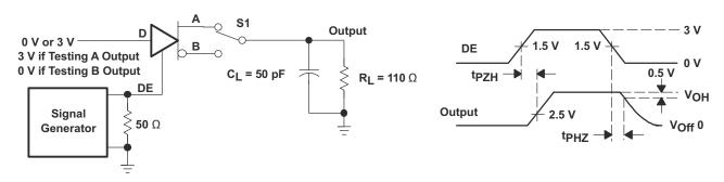
Figure 14. Driver Enable and Disable Test, High Output
