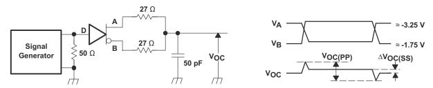
Figure 12. Driver Voc Test Circuit and Waveforms
