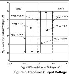
vs Differential Input Voltage
