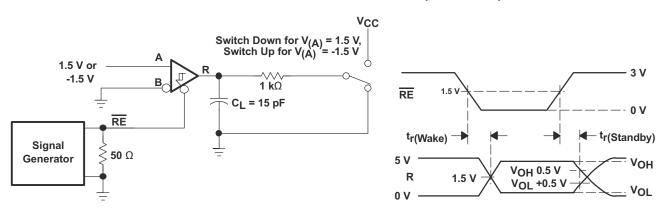
Figure 22. Receiver Standby and Wake Test Circuit and Waveforms
