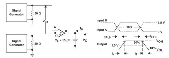
Figure 19. Receiver Switching Test Circuit and Waveforms
