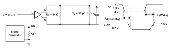
Figure 16. Driver Standby and Wake Test Circuit and Waveforms
