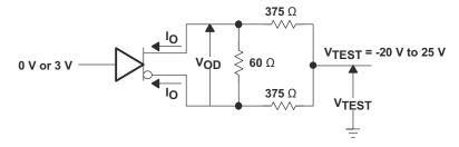
Figure 10. Driver Test Circuit, V<sub>OD</sub> With Common-Mode Loading
