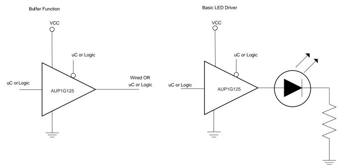
Figure 4. Application Schematic
