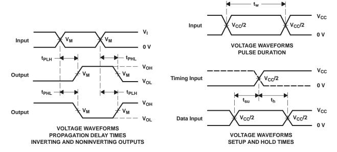
NOTES: A. C<sub>L</sub> includes probe and jig capacitance.
