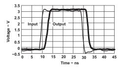
Figure 5. Switching Characteristics at 25 MHz
