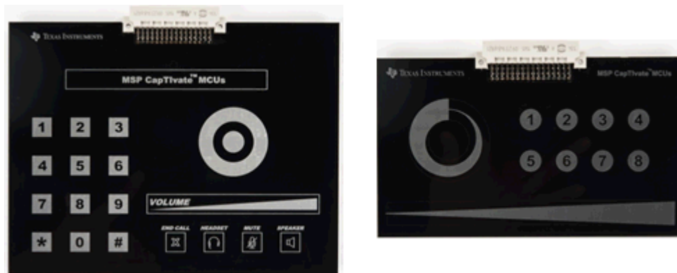
Figure 7-9. CAPTIVATE-PHONE and CAPTIVATE-BSWP Panels
