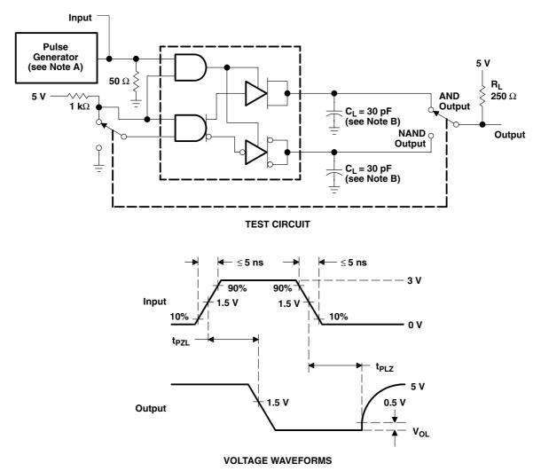
NOTES: A. The pulse generator has the following characteristics:  $Z_O = 50 \Omega$ , PRR  $\leq 500 \text{ kHz}$ ,  $t_w = 100 \text{ ns}$ . B. C<sub>L</sub> includes probe and jig capacitance.
