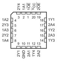
These devices are organized as two 4-bit line drivers with separate  $\overline{OE}$  inputs. When  $\overline{OE}$  is low, the devices pass inverted data from the A inputs to the Y outputs. When  $\overline{OE}$  is high, the outputs are in the high-impedance state.
