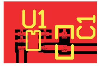
Figure 14. TMP20 Layout with Proper Electrical and Thermal Connections for Pin 2
