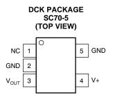
Note: NC or no-connect pin must be grounded or left floating.
