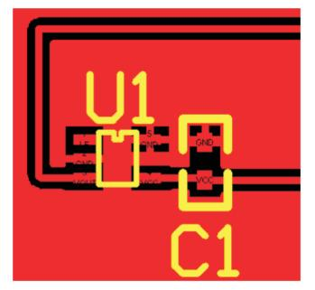
Figure 15. TMP20 Layout with Proper Electrical and Poor Thermal Connections to Ground
