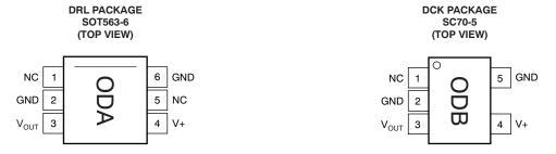
Note: NC or no-connect pin must be grounded or left floating. Pin 2 on the DRL package has no internal connection; pin 2 on the DCK package is connected to the die substrate. See Layout Information for more information about optimizing the connection of pin 2 on the DCK package for thermal and electrical performance.
